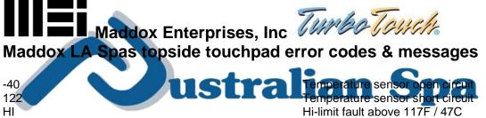
HI / temp display – alternating J11 J12 PSC PSO Flashing 'heat' light Hi-limit fault above 117F / 47C Over temp above 112F / 44C Temp sensor plugged in Jack 11 is faulty or dangling Temp sensor plugged in Jack 12 is faulty or dangling Pressure switch closed Pressure switch open Hi-limit fault on older units – reset with light or pump key
